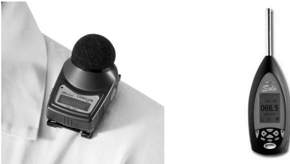
Figure A-6: Dosimeter attached to shirt (left), and sound level meter (right).
