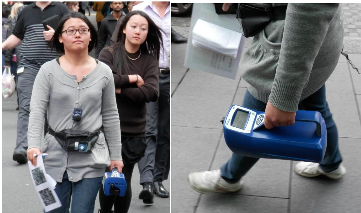
Figure 2-1: A PENAP study participant undertaking mobile monitoring on Queen Street. She holds an ultrafine particle counter, has a carbon monoxide sensor on her belt and a noise dosimeter pinned to her abdomen.
