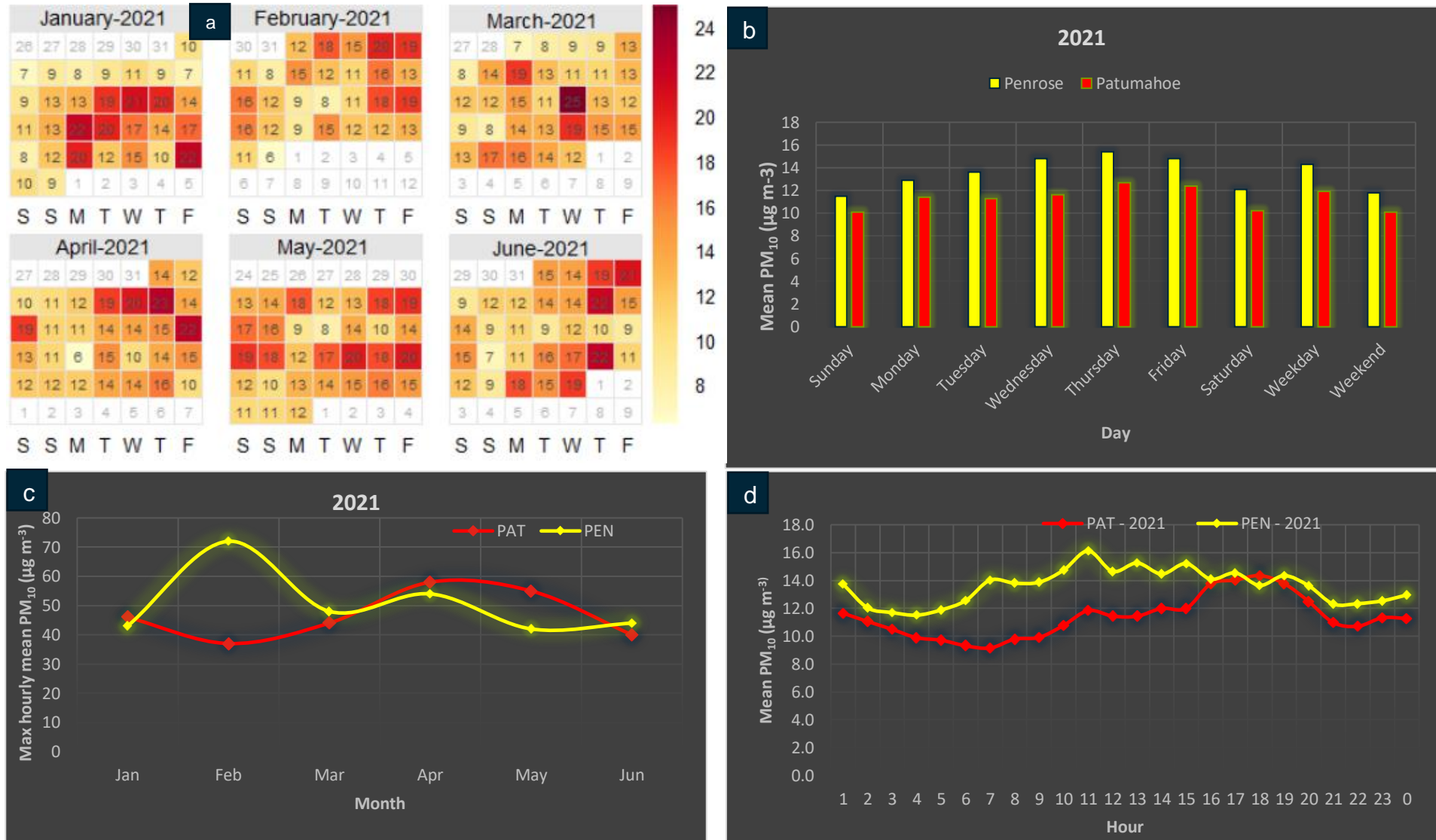
Figure 7. 2021 mean concentrations of PM 10 at Penrose. Plots a , b , c , and d show calendar plot, day, month, and hour variations respectively. Plots b , c and d also shows the comparisons to a rural site. Note: PEN = Penrose, PAT = Patumahoe.
